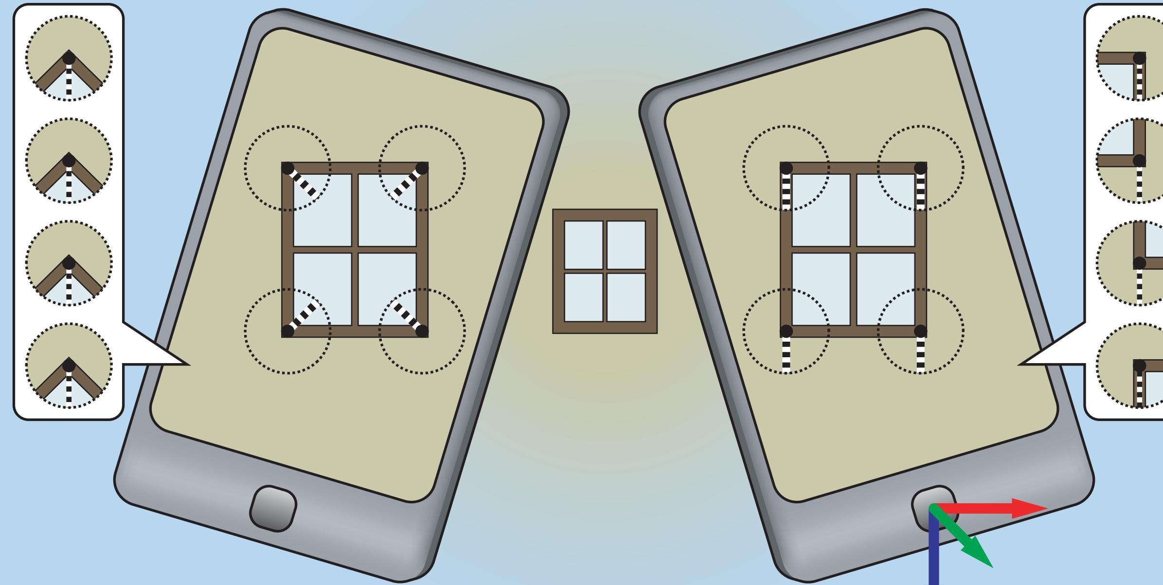
Gravity-aligned feature descriptors (GAFD) use the orientation of the gravity instead of the canonical gradient orientation of a feature.
