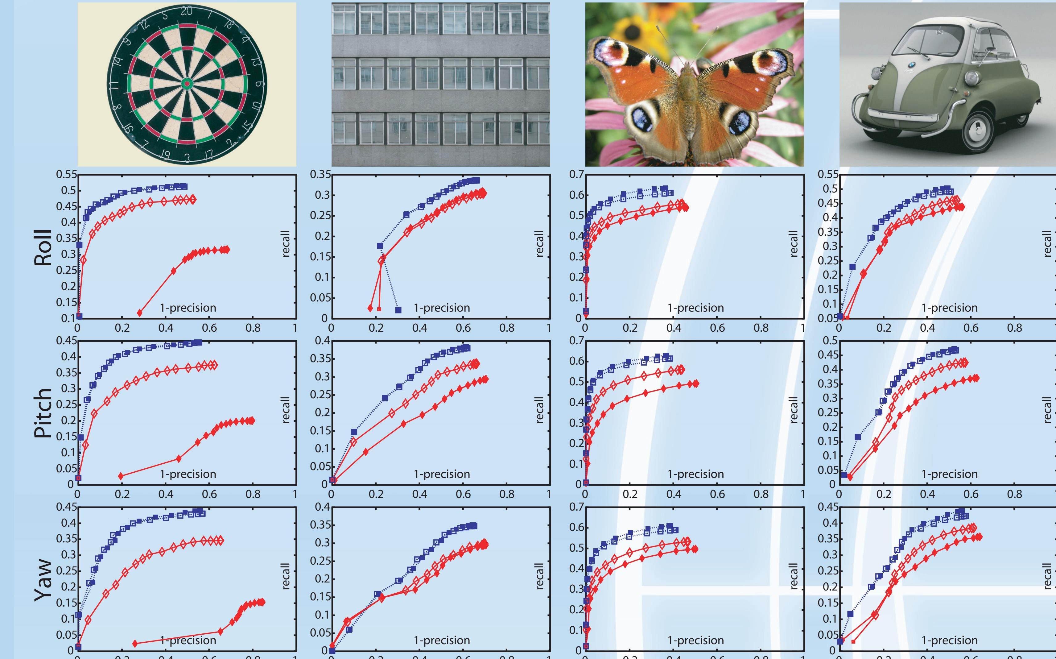
Recall-precision characteristic for different target images under different camera motions. GAFD-SIFT clearly outperforms regular SIFT.
