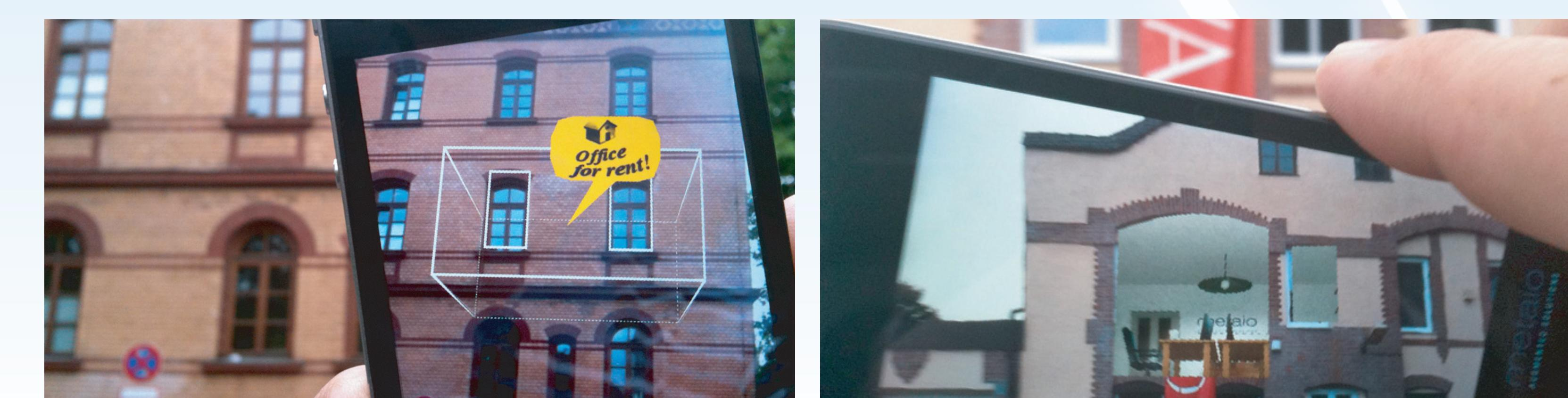
Mobile AR application using GAFD for large scale outdoor tracking.
