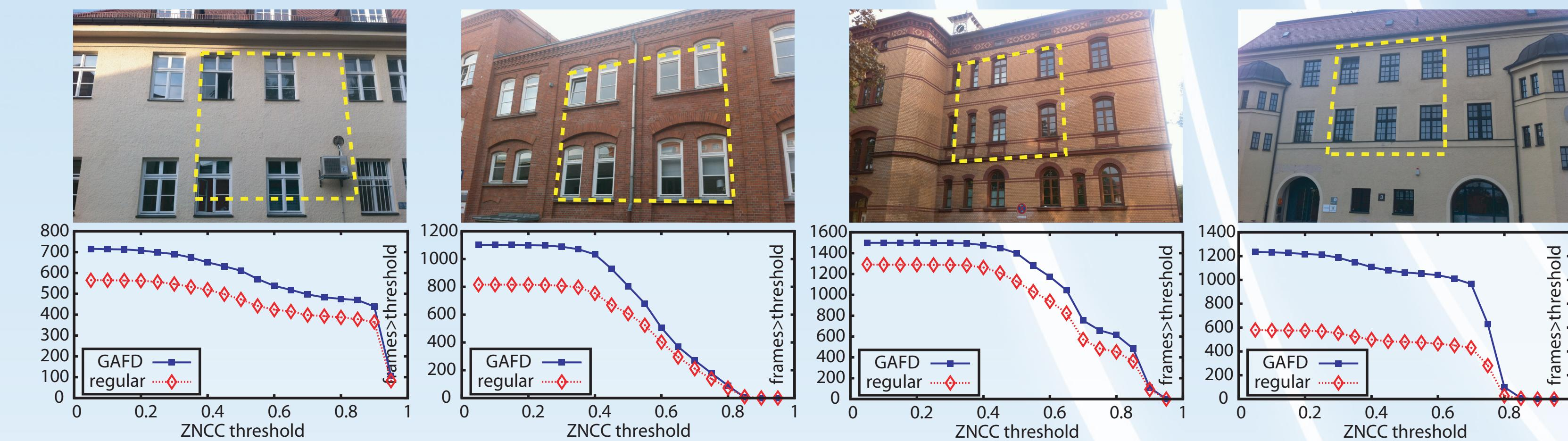
Number of successful detections with respect to the similarity measure threshold: GAFD improves the detection rate.
