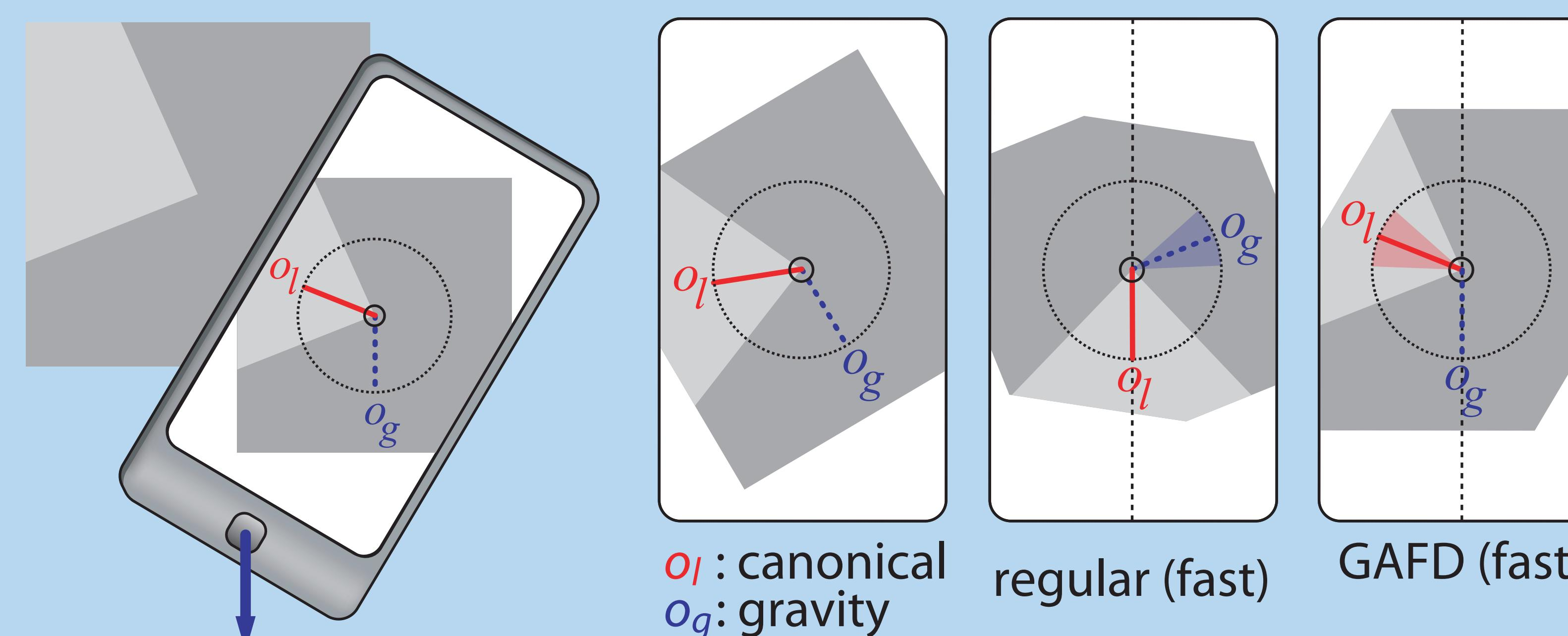
Every feature has a local ( $o_l$ ) and a global orientation ( $o_g$ ). Their difference is constant and can be used to preclude feature matches.
